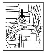
Park the vehicle on a level surface. Check oil only when the engine is cold. Allow the engine to cool two to three hours after running.
